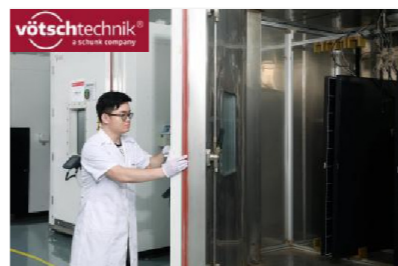
VOTSCH Walk-in Climate Simulation Chamber
